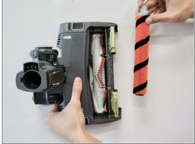
Use the tab on the right side to lift out the soft roller.
