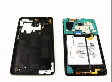
Use the iFixit Opening Tool to pry off the back case, moving the tool around the screen.
