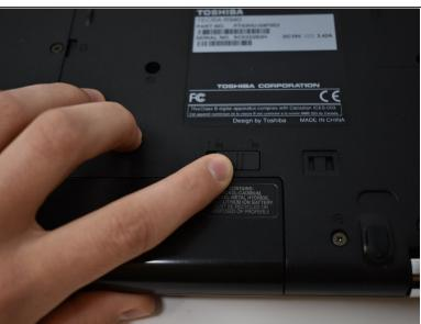
Slide lock 1, located on the right side, to the unlocked position.
