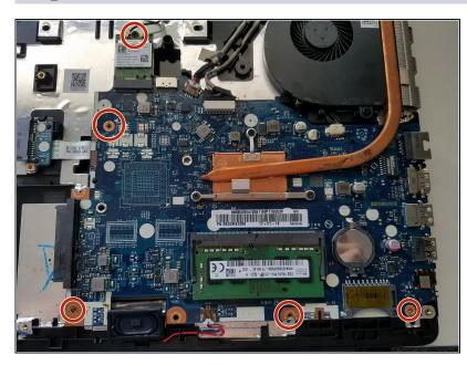
• Using a Phillips #1 screwdriver, remove the five 4.0mm screws.
