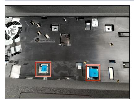
• Pull the two connectors with blue ribbons marked with MB in the opposite direction of the connector
