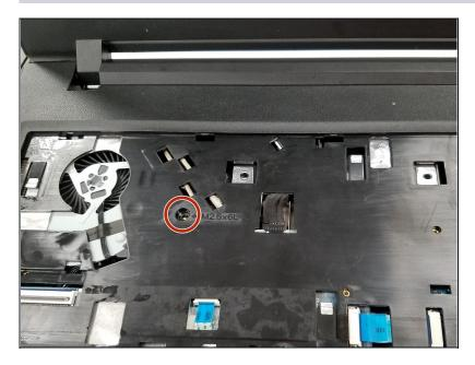
Using a Phillips #1 screwdriver, unscrew the one 5.0mm screw on the back panel.
