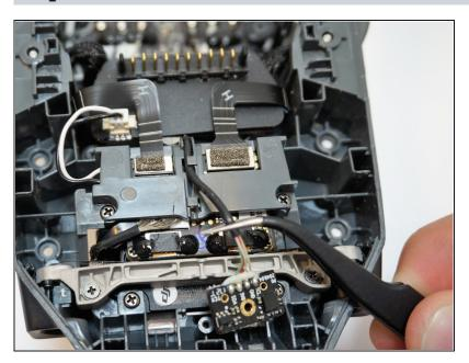
Pull the cord and micro controller board away from the front of the DJI Mavic Pro using tweezers.
