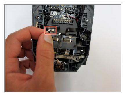
Gently remove the power cable connector located to the left, behind the gimbal board, by pulling up on the white base.
