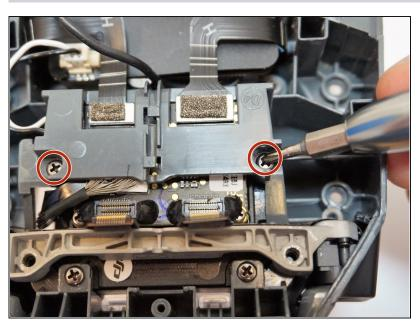
Remove two 6mm JIS #00 screws from the plastic board cover at the front of the DJI Mavic Pro.
