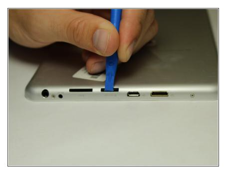
To uninstall the Micro SD Card, push it in using the plastic opening tools until the Micro SD card clicks.
