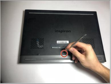
Remove the 3mm screw in the location shown, using a Phillips #1 screwdriver.
