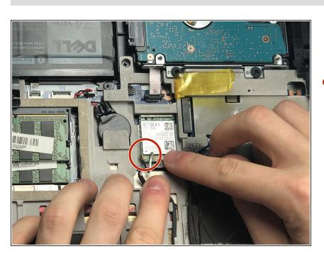
Detach the black and white wires connected to the card by gently lifting up on the wires.
