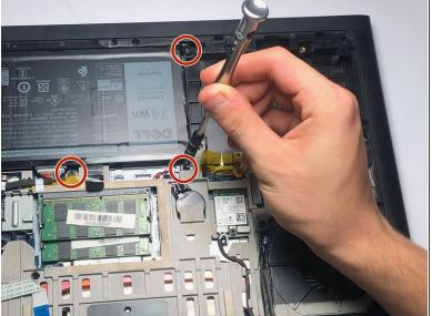
• Remove the five 3mm screws on the battery with a Torx (T8) screwdriver in the locations shown.
