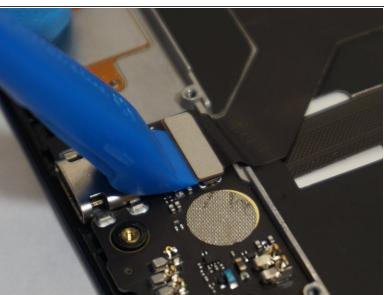
• Use the plastic opening tool to separate the connector ribbon from the bottom center of the phone.
