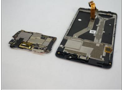
Carefully lift the motherboard out of the frame.
