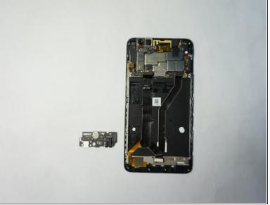
Use the plastic opening tool to remove the charging port card of the phone.
