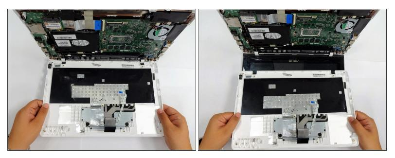
Now that the keyboard connectors are unplugged, pull the keyboard off and away from the back panel hinges.
