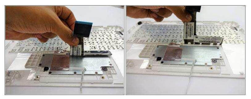
• Lift the keyboard connector from the keyboard.
