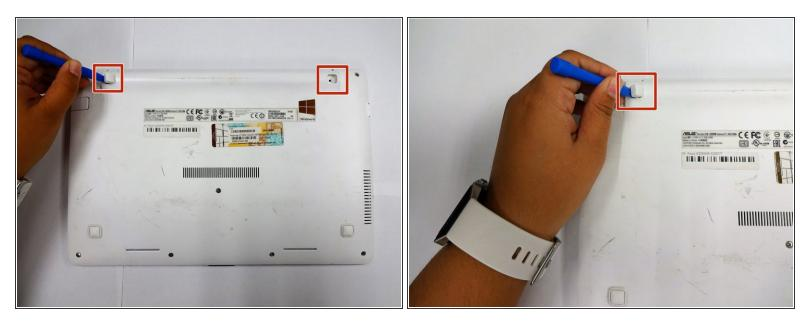
Using a plastic spudger, remove the two rubber stoppers closest to the hinge to reveal the screws underneath.
