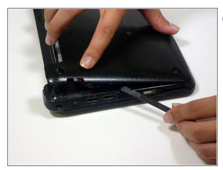
from the netbook easily, use the spudger to pry off the back case by the edge near the battery compartment, and work your way to the sides. The case will then pivot along the front edge.
