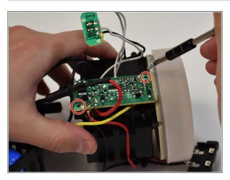
Remove the two 1 mm Phillips #2 screws in the shown locations.
