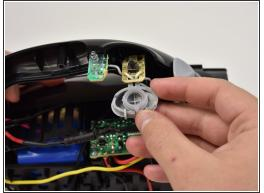
• The power button can be removed by gently lifting it off the circuitry.
