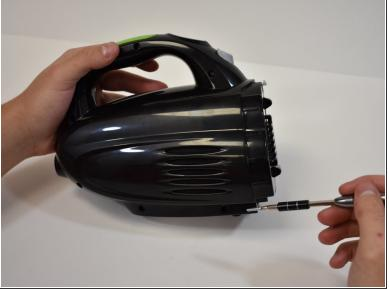
Remove the six 1.2 mm Philips #2 screws from the handle and base.
