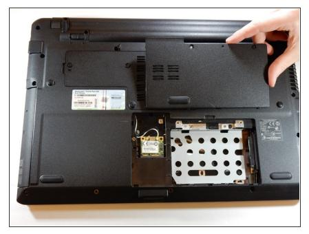
Once you have have removed the back panel cover, find the hard drive's location.
