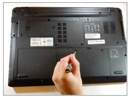
Locate where the hard drive is located on the back side of the laptop and unscrew the two .8cm Long screws.
