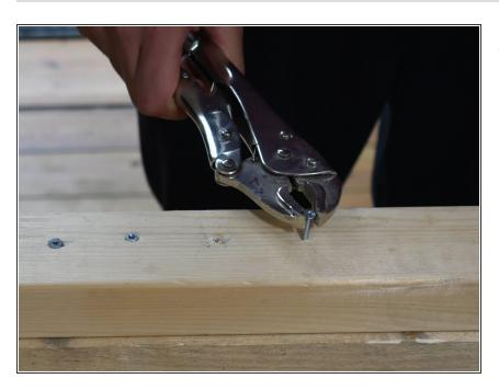
If the screw is protruding then you may be able to use a pair of locking pliers.
