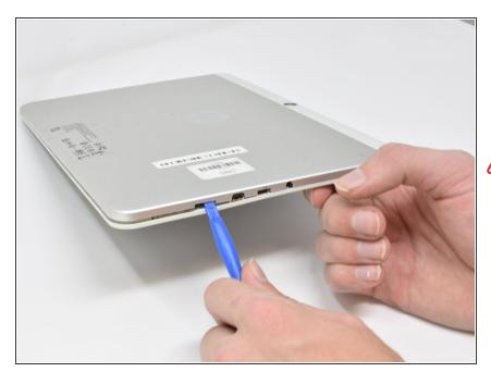
Insert the smallest plastic opening tool into the SD card port. Gently pry until the back panel separates from the screen panel.
