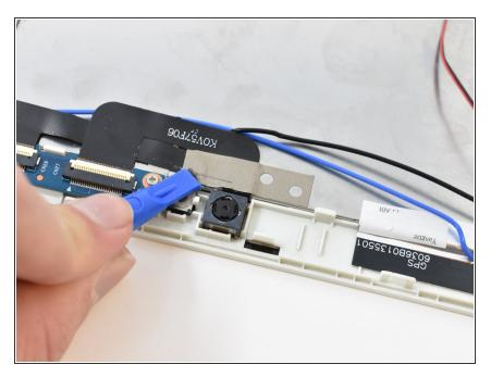
• Peel off the metal mesh tape with the plastic opening tool.
