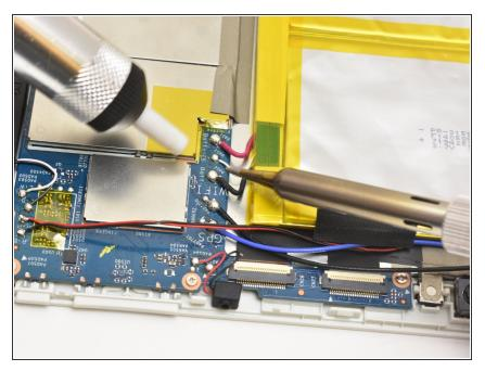
• Desolder the battery connectors from the motherboard.
