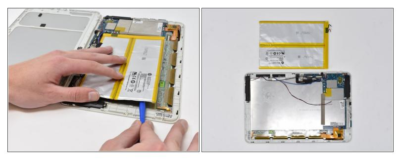
• If the previous step is unsuccessful, wedge the smallest plastic opening tool between the adhesive and the metal display casing.
