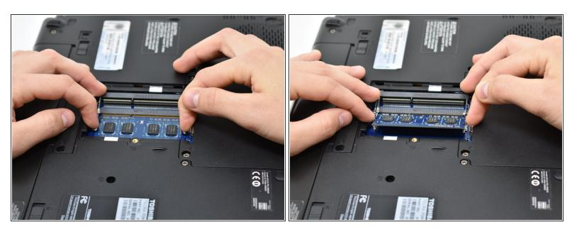
Repeat the previous step of pulling the RAM card out for the second card, but using the lower brackets.
