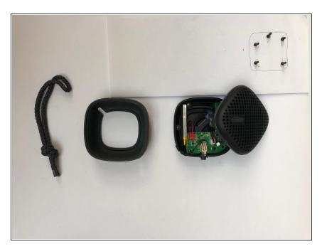
Removing speaker grill, undoing 5 screws on the back. Using PH1 Screwdriver.
