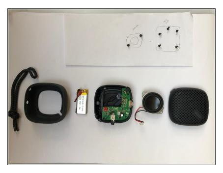
Removing speaker carefully undoing clip on the circuit board.
