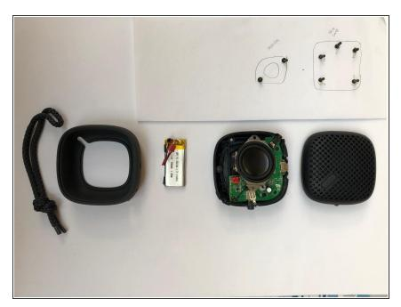
Removing battery carefully undoing clip on the circuit board.
