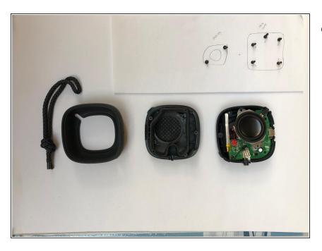
Undoing 2 Screws using PH1
