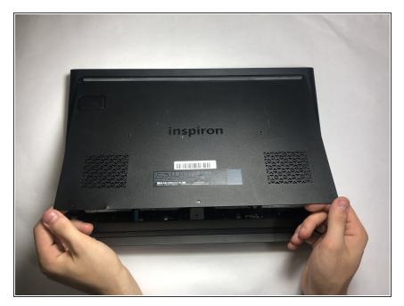
Remove the panel from the sides and pull it out at an angle towards you.
