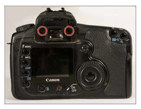
Remove the two screws hidden under the viewfinder eyepiece cap.
