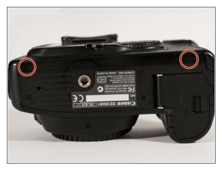
Remove the two indicated screws from the bottom of the camera.
