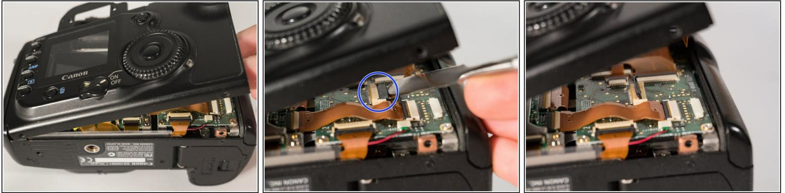
**⚠** When lifting the panel, make sure not to lift it too high, since you'll run the risk of tearing the cable, or damaging the connector on the board.
