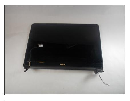
• Remove the LCD display assembly from the laptop.
