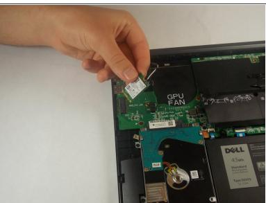
Remove the Wifi-Card from its socket by pulling away and up from the connector.
