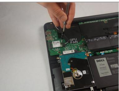
Remove the 3.0 mm-long Philips #0 screw at the end of the Wifi-Card
