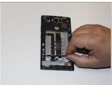
Use a plastic opening tool to lift the charging port circuit board.
