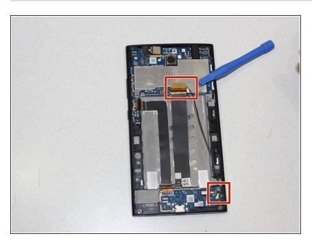
Unhook the antenna from circuit board using a plastic opening tool and remove the charging port circuit board from the device.
