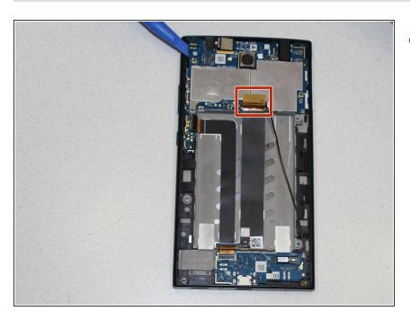
Unclip circuit connectors from phone to motherboard.
