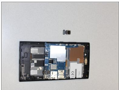
Detach the rear camera from motherboard and remove it from the device.
