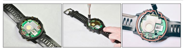
• Use a T5 screwdriver to remove the two silver 1.4 mm screws from the motherboard.
