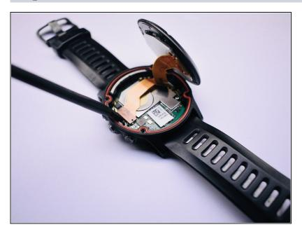
• Use a spudger to lift up and free the screen ribbon cable's press-fit connector from the motherboard.
