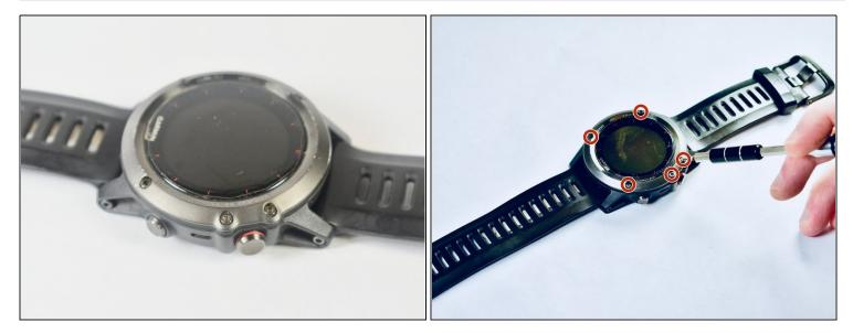
• Use a T6 screwdriver to remove the five 1.7 mm screws from the watch face.
