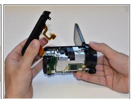
• Grasp the top of the camera and pull straight up to remove the top panel.
