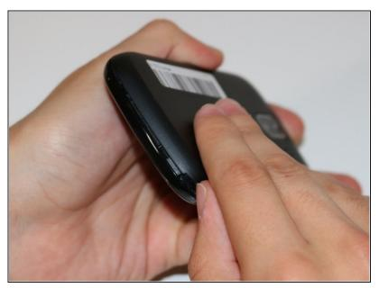
• In the bottom right corner of the device, use your fingernail to remove the back cover of the phone by lifting up and holding the device with your other hand.
