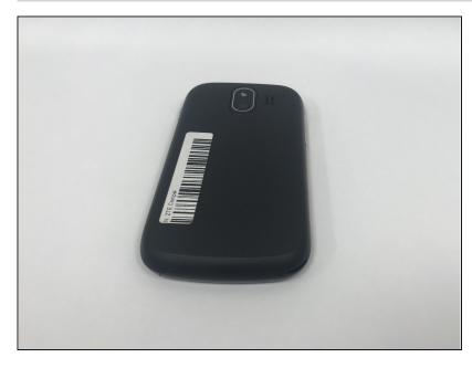
Place the phone on a flat surface with the screen facing down. This will allow easy access to the removable black plastic cover on the back of the phone.
