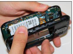
• Insert the flat end of your black plastic spudger into the crease and work it around the entire circumference of the phone until the front and back are separated.
