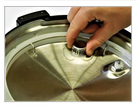
Securely grasp the steam release valve cover. Twist and pull firmly to remove the valve cover.
