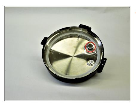
Flip the lid over to expose the underside and the steam release valve cover.
