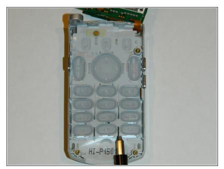
While avoiding contact with the inner electronics, use the spudger to lift the plastic keypad from the phone.
