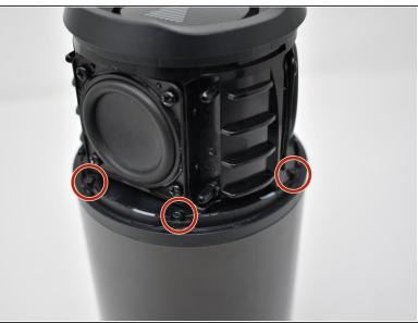
Use a Phillips #00 screwdriver to remove the six black 6mm screws on the inside of the top of the bottom section.
