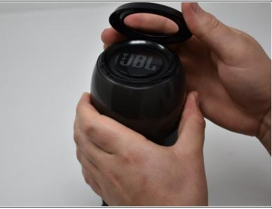
Turn the JBL Pulse 3 right-side up and unscrew the top ring of the device. A small amount of force and/or a cotton cloth may be necessary to remove this piece.
