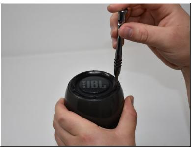
Remove the six 5mm screws on top of the JBL Pulse 3 with a Phillips #0 screwdriver.
