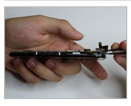
Use your tweezers to disconnect the final ribbon connector underneath the motherboard at the top of the phone. The motherboard can now be separated from the LCD Screen. To reassemble your device, follow these instructions in reverse order.
