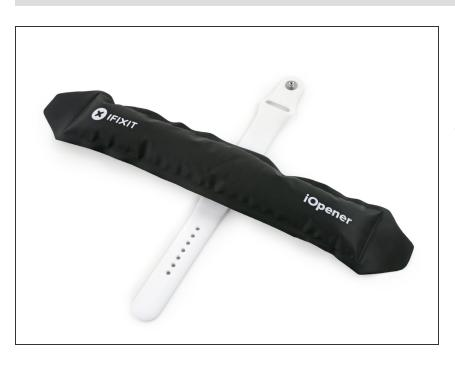
Microwave your iOpener for another 30 seconds, and apply it to the front of the watch case to soften the adhesive securing the Force Touch sensor.
