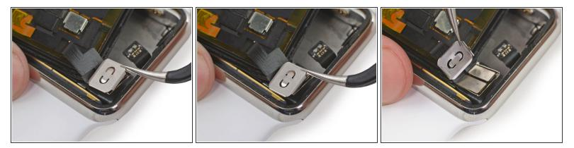
Grab the cover with your tweezers and slide it toward the top of the watch to free the final slotted tab, and remove the cover.
