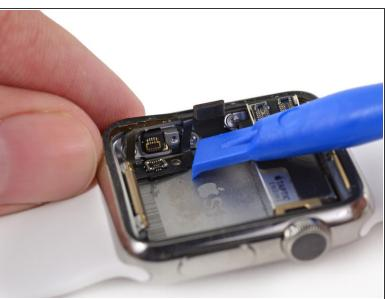
Use a plastic opening tool to flip the Force Touch sensor cable connector straight down, disconnecting it.
