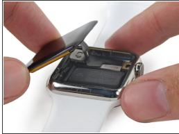
Lift the screen up and shift it to the left, minding the display data and digitizer cables.
