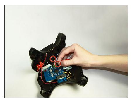
If transmitter has broken or has disconnected wires it may need replacement. Wires can easily break loose from the transmitter. The wires can easily be reinserted by sticking the wire back into its original slot.
