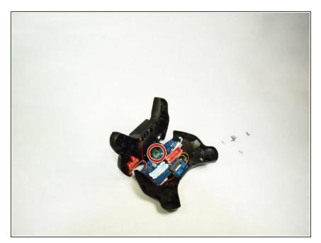
With the circuits exposed locate the transmitter at the top of the controller. It is green hue in comparison to the rest of the blue circuits. Check the transmitter for damage or disconnected wires.
