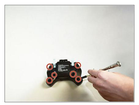
Locate and remove the six screws on the back of the controller.
