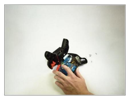
With the controller facing down remove the top casing from the bottom. Do this by popping the casing lose which will expose the inside circuits.
