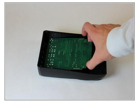
• Lift the indented end of the motherboard opposite the input/output jacks. Then, pull away from the input/output jacks to slide the motherboard out of the casing.
