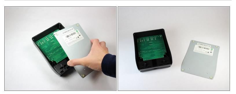
• Remove the back panel to expose the motherboard.
