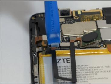
• Using a plastic opening tool, separate the fingerprint ribbon connector from the motherboard.
