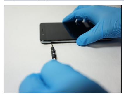
Remove the one T2 screw from the side of the phone near where the SIM card tray was.
