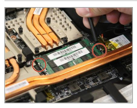
Pop the metal tabs on each side of the RAM using the black nylon spudger.
