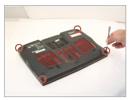
Unscrew each of the four screws using the Phillips #0 head on the back of the laptop case. The screws are 0.5 inches in length.
