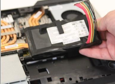
Pry the battery pack up with the black nylon spudger.
