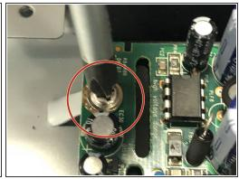
unscrew two screws at the back of the body and one on the board, then lift the circuit board away from the main body.
