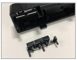
unbent the metal piece holding the front shell and pull it out, take off the button circuit and the push button component.
