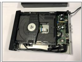
Take off these two black screws at the edges and lift the top shell of the main body.
