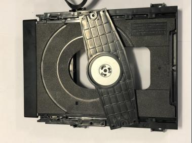
unscrew the two screw that holds the cover and lift the cover away from the loader.
