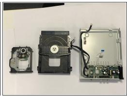
unplug the cable connecting the laser lens and the main circuit and lift the laser lens away from the main body.
