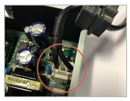
unplug the power cable from the main circuit board.
