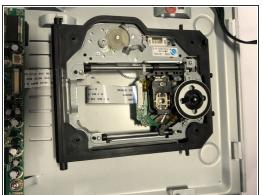
• unplug all cables from the main circuit and lift the loader from the body only leaving the laser lens.
