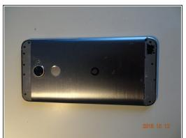
To open the device you need do apply pressure at the bottom and up to get rid of the glued mini covers.
