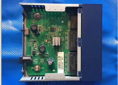
• Use gentle pressure to pull back the top and rear panel of the switch away from the body and set side.
