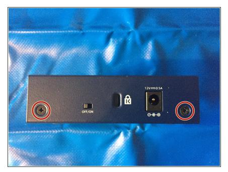
Remove the two 4.04 mm Phillips Head screws with a PH1 bit or Phillips #1 Screwdriver and set screws aside.
