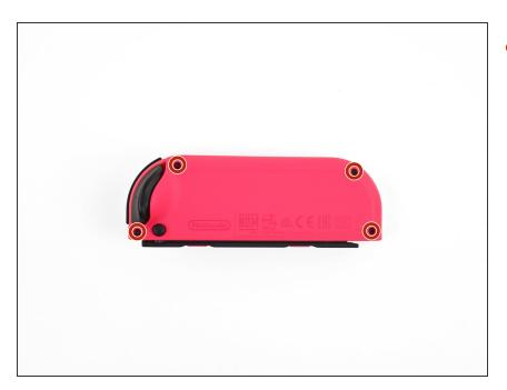
Remove the four Tri-Point Y00 screws from the back panel of the Joy-Con.
