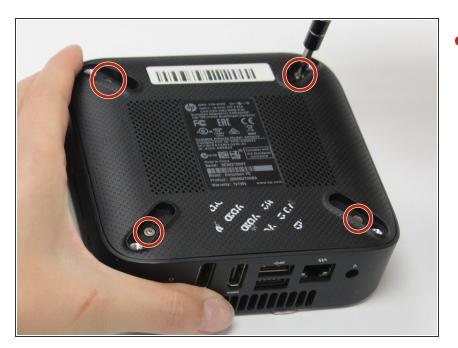
Using your Phillips head screwdriver, remove the four Phillips M2.5×4.0 screws that secure the bottom cover to the computer. In this step the usage of the magnetic mat will be helpful to keep up with the screws.
