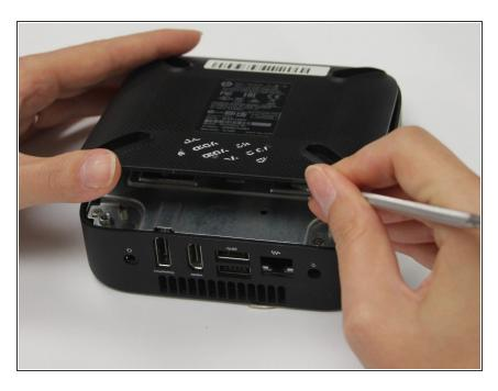
Insert the flat end of your metal spudger under the bottom cover near the USB ports, then pry the bottom cover off the computer.
