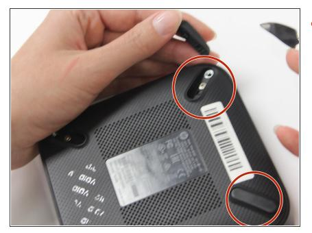
Using your metal spudger, lift and remove the 4 rubber "feet" from each corner.
