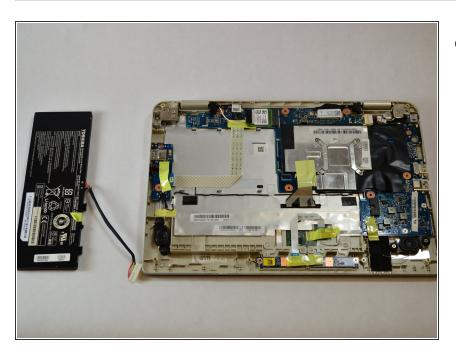
Carefully unplug the battery from the device motherboard.
