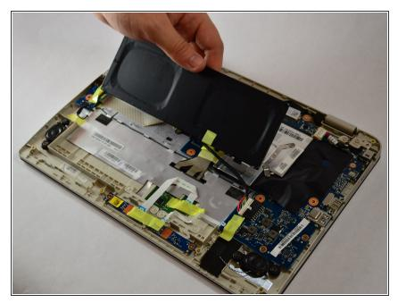
Lightly grip the battery on the two longest sides. Gently pull up until the adhesive on the notebook is separated from the battery.
