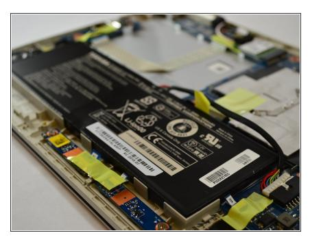
Remove the 1" yellow tape on top of the battery. This piece of tape is holding down the battery connection cable.
