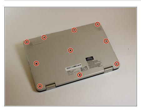
Unscrew the 10 5mm Phillips screws, located on the bottom side of the notebook using the PH1 bit and the Magnetic Driver.
