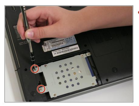
Use a #0 Phillips screwdriver to remove the two 4.0 mm screws attaching the hard drive to the laptop.
