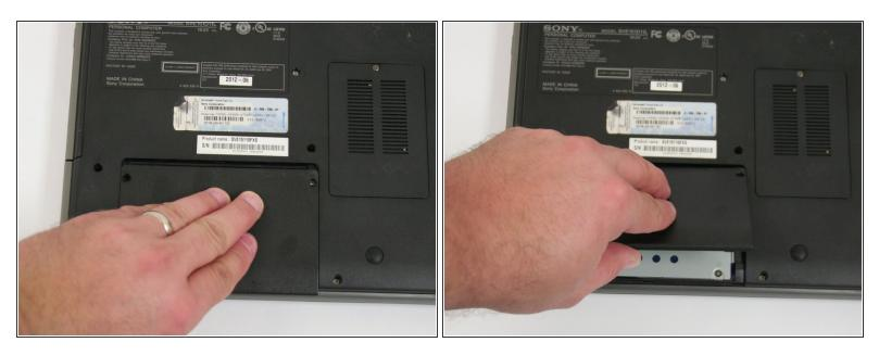
• To expose the hard drive, remove the cover by sliding it toward you and pulling up on the panel.
