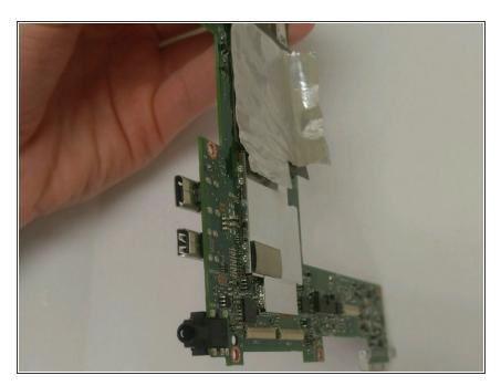
Remove the motherboard from the device.
