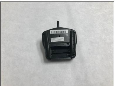
Remove the batteries (2 AA).
