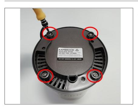
Unscrew the four 10mm screws (located in the red circle) with the Philips head #1.
