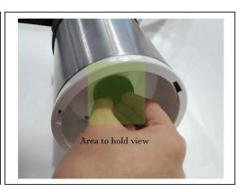
• Firmly hold the top section of the rotator up (indicated in the green section), while firmly using the other hand to unscrew the internal screw with a #1 Phillips head (located in the red circle section). Continue this process until the two parts are separated from the main component.
