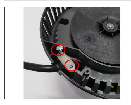
Unscrew the two 10mm screws (located in the red circle) with the #2 Phillips head. When all screws are separated from the main body, without effort, detach the plastic component off the appliance.
