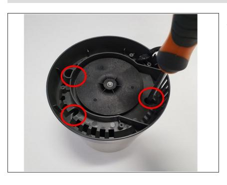
Unscrew the three 13mm screws from the base with the #1 Extended Philips head screwdriver.
