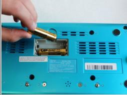
With the battery panel off, remove the batteries. Use your hands or a plastic spudger to remove the batteries.
