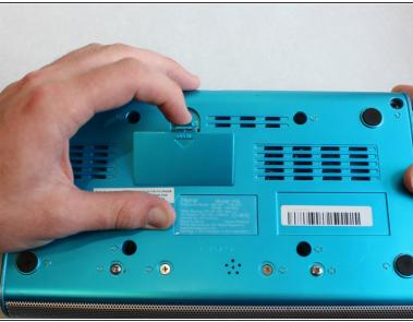
• Using your finger, pry the tab on the battery cover to remove the battery cover on the back of the iHome to access the batteries.
