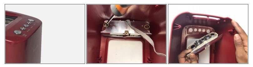
• Unfasten the two Pan Phillip head screws to detach the buttons' housing
