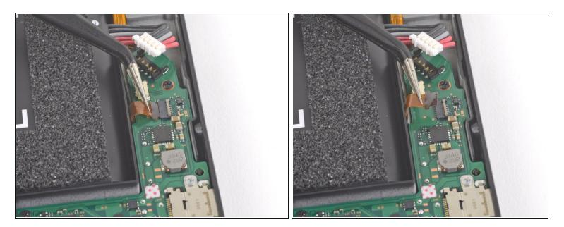
Use a pair of tweezers to slide the Joy Con rail data cable straight out of its connector on the motherboard.
